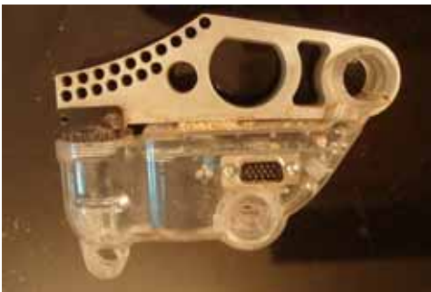
This is the Brake that stops the blade.
