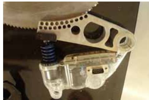
This shows the brake after it has engaged with the blade. The brake and the blade are both sacrificed and must be replaced but the finger is still intact.
