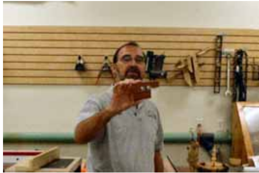
Floyd Yoder – Made his own moulding to restore a chair he is working on. Moulding was made using a custom made scratch stock held by wooden handle. Floyd finally found a use for his bent sawsall blades.
